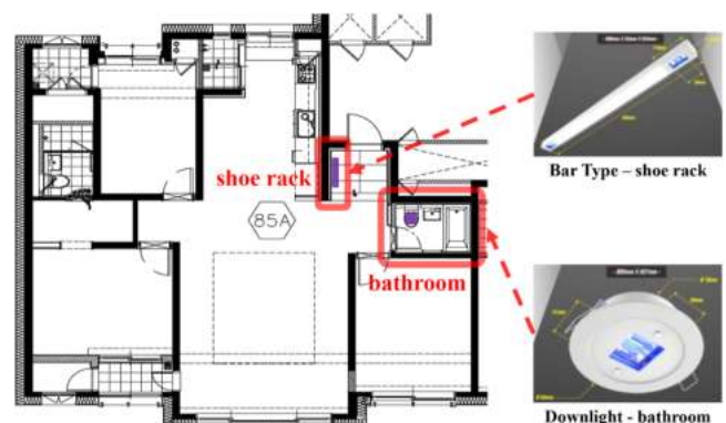
Fig. 1. Plan of target space and far-UVC (222 nm) module location.
