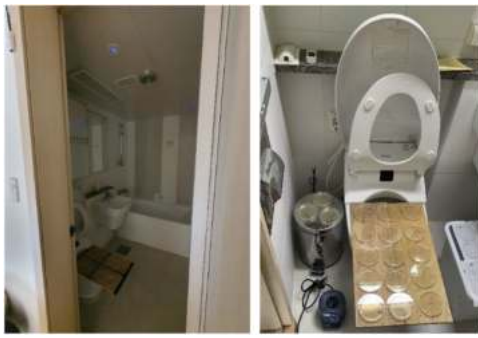
Fig. 6. 222 nm LED module on the bathroom. (a) Far-UVC module in the bathroom. (b) Measurement on the toilet.
